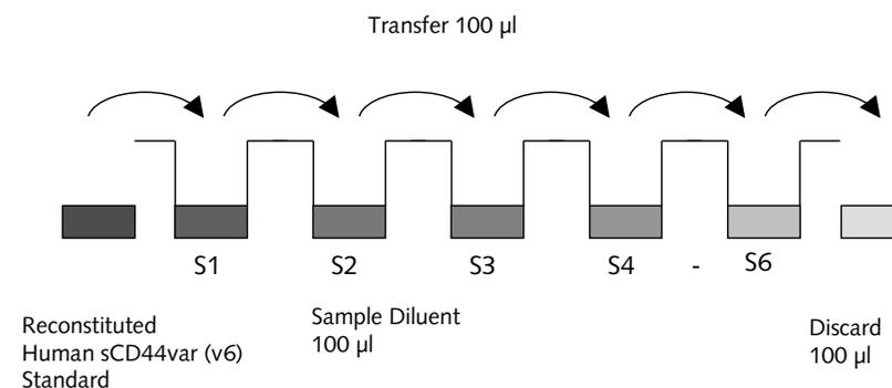
In case of an **external standard dilution** (see 9.4.1.), pipette 100 µl of these standard dilutions (S1 - S6) in the standard wells according to Table 1.
