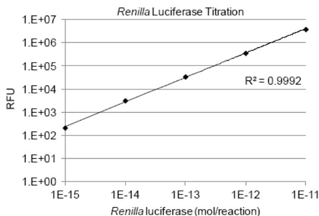
**Figure 2.** Titration of recombinant Renilla luciferase in the PromoKine *Renilla* Luciferase Assay. *Renilla* luciferase was serially diluted in 1X Passive Lysis Buffer and measured in the assay. Luminescence was measured on a Promega Glomax® 20/20 single tube luminometer with integration time of 1 second. Background from reagents without enzyme added was subtracted from luminescence values.
